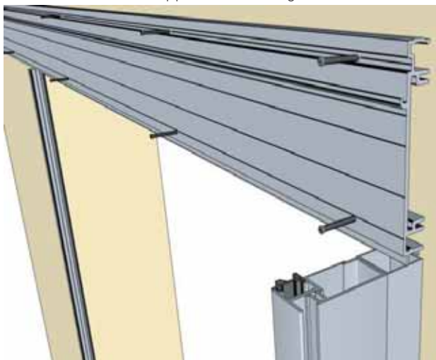
Support beam fixing
